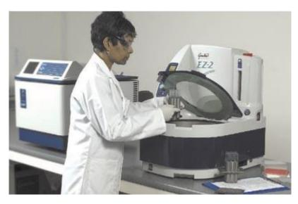
The recent introduction of an EZ2 centrifugal evaporation system for clinical biochemistry sample preparation has provided this particular hospitals laboratory staff with considerable advantages compared with the manual dry down evaporation methods previously used.
